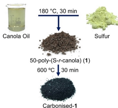
Figure 1. A sulfur-rich graphitic carbon was prepared from a sustainable polymer made by the direct copolymerisation of sulfur and canola oil.
